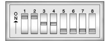
Example of Eight Dip Switches with Three Positions
