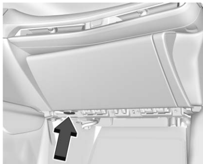
Interior Power Outlet
